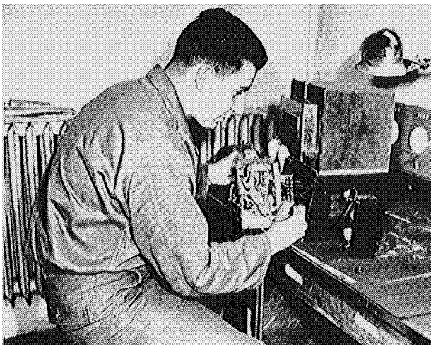
Pvt. Ysais check the electrical connections of Dental Furnace.
